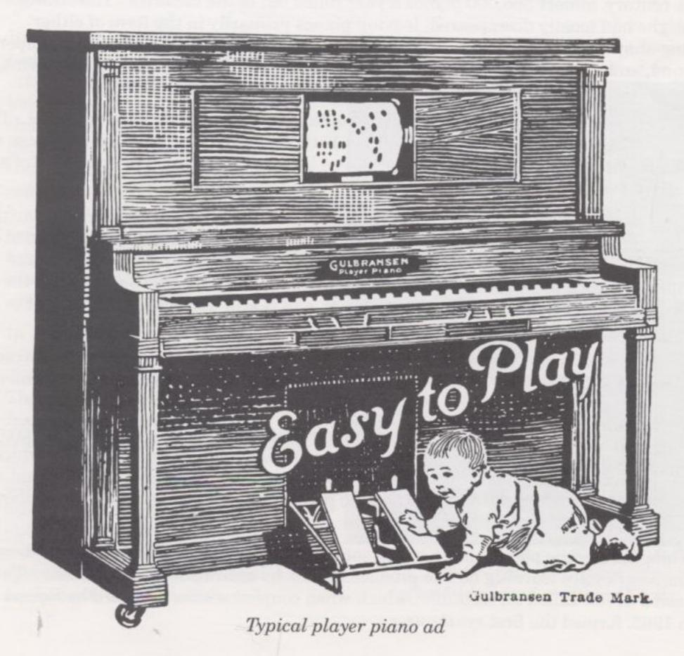
Perhaps the most unique of these inventive pianos was the one that required no pianist. The *player piano* could duplicate a performance by rolling a hole-punched sheet of cardboard past a line of air jets, one for each key. Each hole represented one note of the performance. When a hole passed a jet, the air shooting through it would fire the appropriate hammer at the piano's strings.
